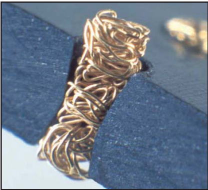
Connector Cross Section Showing CIN::APSE® Contact
